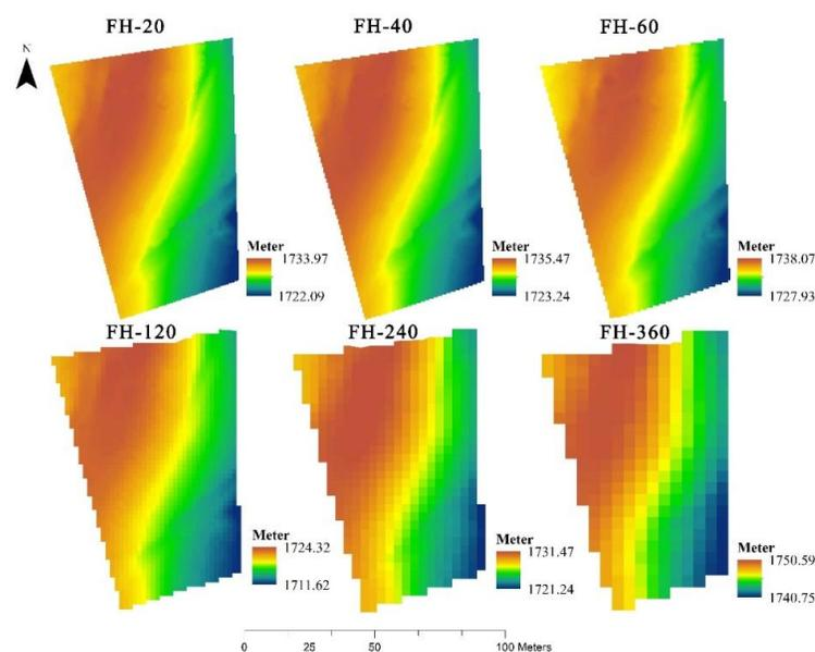
**Fig.2: multiscale DSM obtained from image acquisition and processing.**
