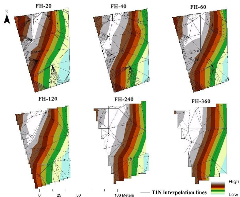
**Fig.4: TIN models of contour surface at the six flight heights.**
