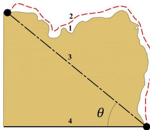
**Fig. 1** The rugosity of a surface (e.g. yellow profile of a terrain № 1) is the ratio between the contoured distance (dashed line № 2) and the planar distance (or area for three-dimensional data).
