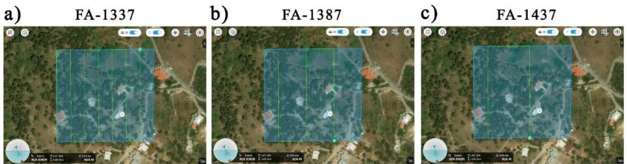
Fig-2. Flight paths designed in Dji ground control flight planning mobile application. Flight rectangle is approximately 196 x 180 m which represents a single flight sequence. a) flight path of 1337 m altitude, b) flight path of 1387 m altitude, c) flight path of 1437m altitude.
