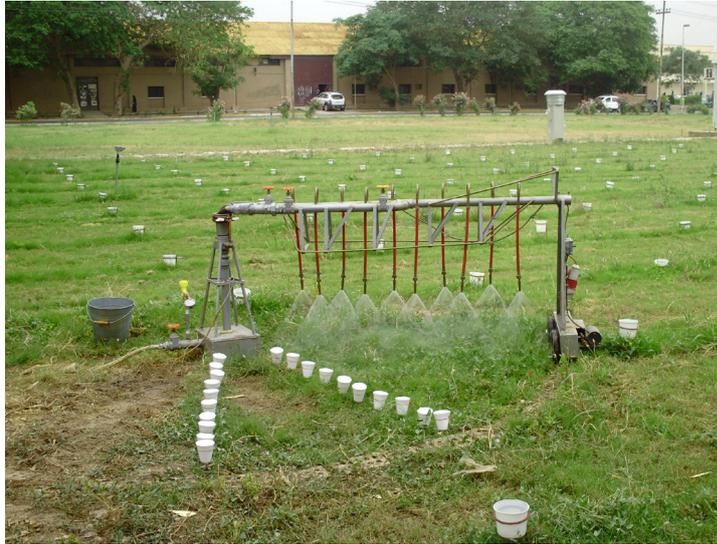
Fig. (2). The catch containers setting with the physical model of center pivot system
