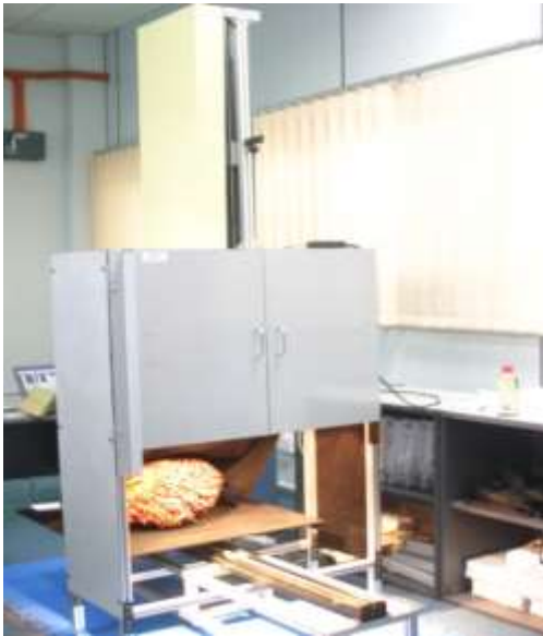
Figure 5 Schematic view of the hyperspectral imaging system showing the bunch on the conveyor
